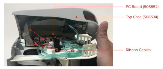
6. On the PC Board (508552), disconnect the wires that go to the O2 Sensor (508419), dose valve (518166), and crossover valve (508568).
