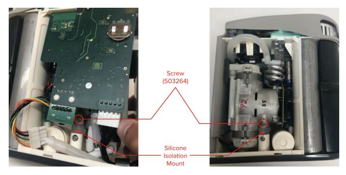
8. Remove the compressor assembly (508525) from the silicone isolation mount (508554).
