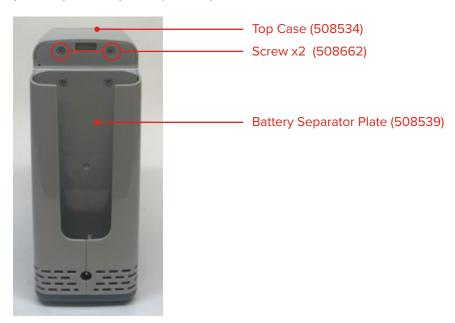
2. Carefully turn top case (508534) toward PC board (508552) and remove the 2 ribbon cables from the PC board.
